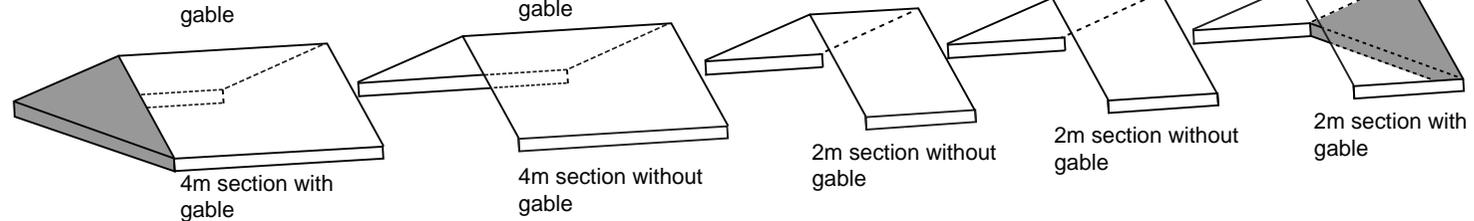
When you are making your CombiTent **shorter**. Use the velcro overlay to detach roof sections.
