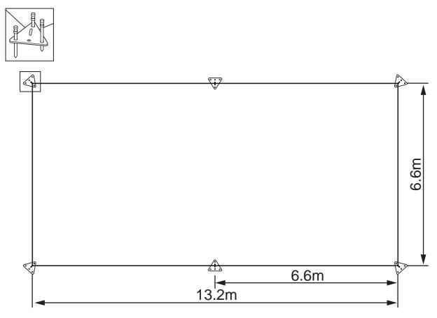
3. Spread a ground cloth over the area defined by the baseplate. Unroll the tent roof, with top side up from the center of the covered area.
