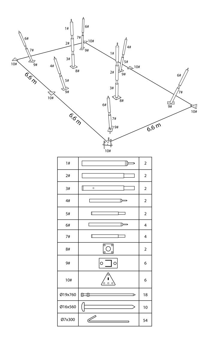
1. Find correct dimension by measuring the distance as follows. Start from one spot, and then measure and find the rest of the spots (six in total). Use Stake Ø7x300 to mark the spots.
