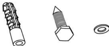
Φ10×50 anchor bolt, M8×75 hexagon wooden screw, Φ8 washer (x4 pcs)
