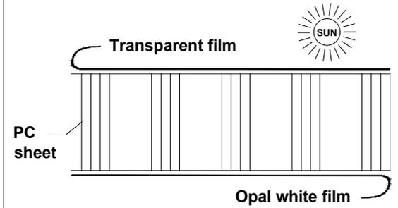
Two sides of PC sheet are covered with thin film, one side's film is transparent, another side's film is opal white. The UV-protected side of PC sheet is covered with transparent film and must face towards the sun.
