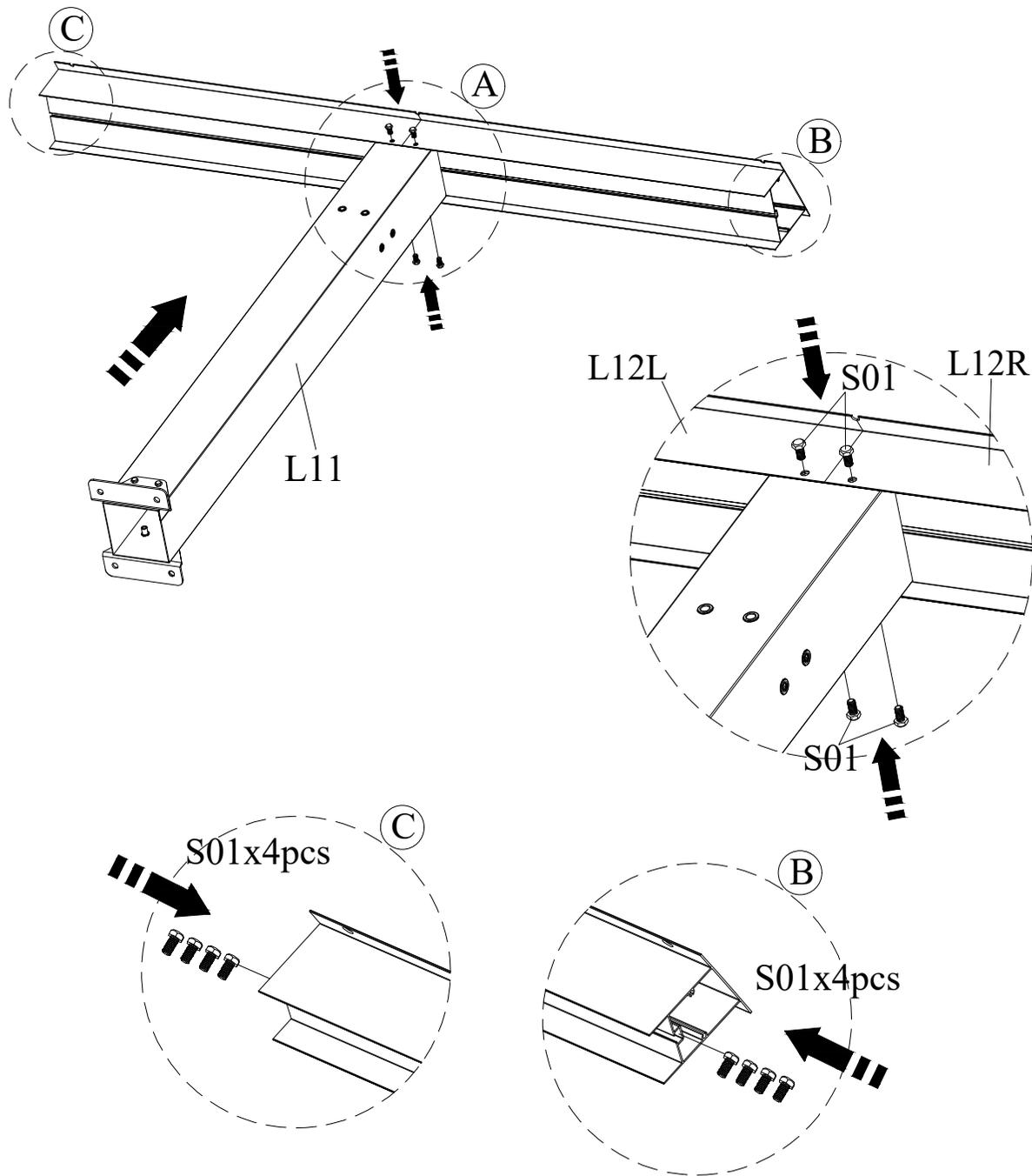
There are 2 assembling holes on this side of L11, see page 13 to assemble W18.
