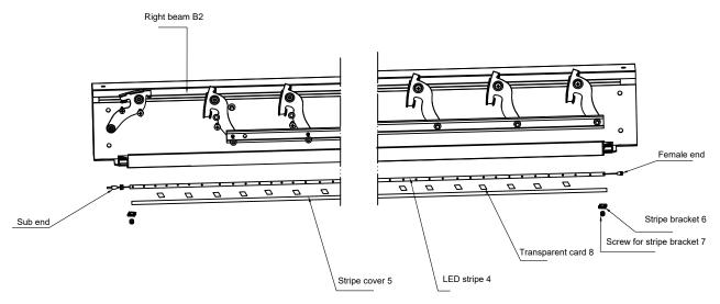
Step 3: Install the LED stripe 4 onto the left beam B1
