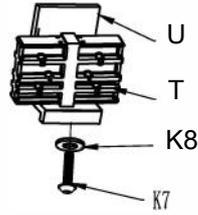
Step 1. Attach the middle connector T to the middle wall base U with screw K7 and spacer K8, taking care not to tighten screw K7.
