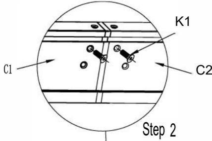
Step 2. Insert front and rear beams C1/C2 into middle connector T respectively and connect them with screw K1, then tighten K1.
