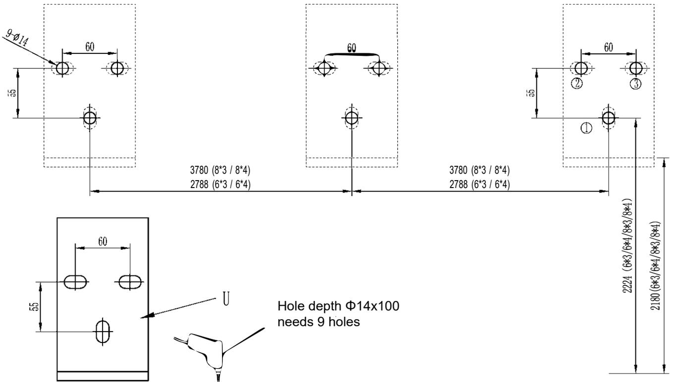
Step 2: Install another two wall brackets U same way, then put on M10 screw and covers K11.
