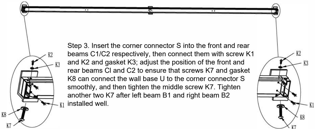
Step 3. Insert the corner connector S into the front and rear beams C1/C2 respectively, then connect them with screw K1 and K2 and gasket K3; adjust the position of the front and rear beams C1 and C2 to ensure that screws K7 and gasket K8 can connect the wall base U to the corner connector S smoothly, and then tighten the middle screw K7. Tighten another two K7 after left beam B1 and right beam B2 installed well.
